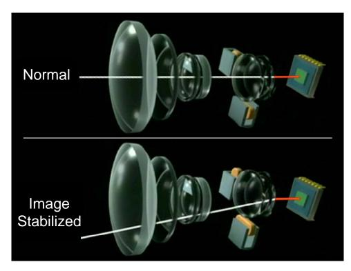
Mechanism of image stabilization
