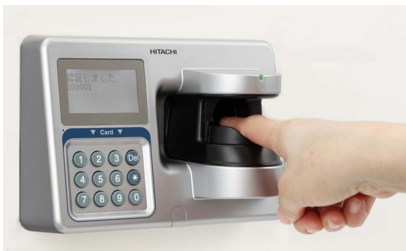
Finger vein authentication system used for the control of entry to facilities
