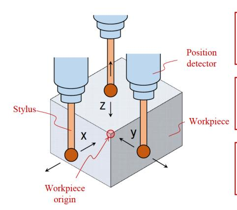
Setting a corner of a workpiece as the workpiece origin using a position detector to indicate the positions of the tool, workpiece and other objects in coordinate values
