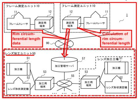
The measurement terminal of the frame measurement unit calculates the rim circumferential length and transmits the rim circumferential length data to the lens edging unit (Element B2/C3, Specification 0017/ 0019)
