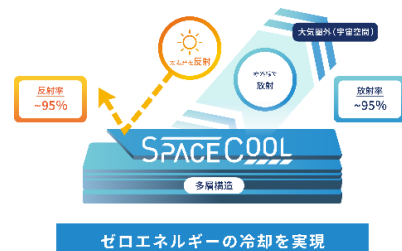
SPACECOOL の放射冷却原理イメージ Concept Image of SPACECOOL's Radiative Cooling Principle
