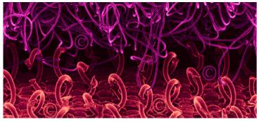
Colorized scanning electron micrographic image of joined VELCRO<sup>®</sup>. © Dee Breger, Drexel University
