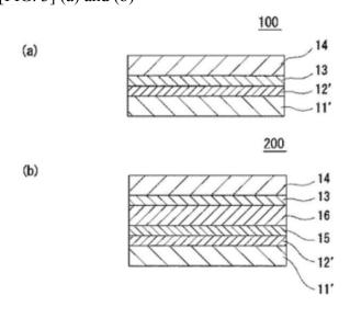
An optical film laminate 100 has a thermoplastic resin substrate 11', a polarizing film 12', a pressure-sensitive adhesive layer 13, and a separator 14, in the stated order. An optical film laminate 200 has the thermoplastic resin substrate 11', the polarizing film 12', an adhesive layer 15, an optical function film 16, the pressure-sensitive
