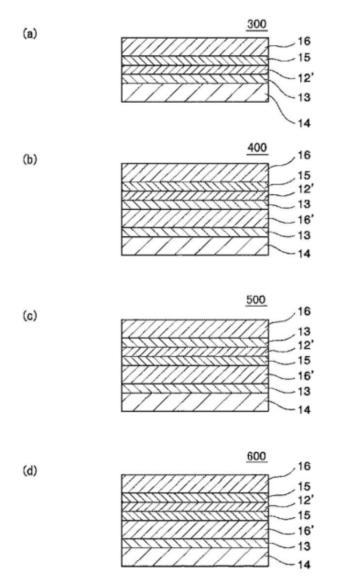
An optical function film laminate 300 has the separator 14, the pressure-sensitive adhesive layer 13, the polarizing film 12', the adhesive layer 15, and the optical
