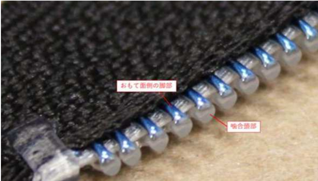
おもて面側の脚部 Leg section on the front surface side 啮合頭部 Engaging head section
